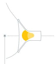
For a good fit, the nipple should be centred within the breast shield tunnel, with space to expand and move freely.
