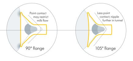
By testing wider-angled flanges, the researchers found 105° better matched the contours of the scanned breasts, regardless of shape or size. In addition, the nipple was placed further into the tunnel and point contact was reduced at the rim – suggesting a more comfortable pumping experience for mothers, and the possibility of improved milk flow.<sup>4</sup>
